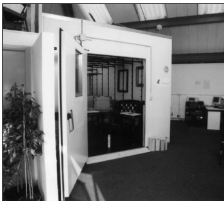
The sealed chamber uses lower temperatures and inert gases to eradicate pests.
