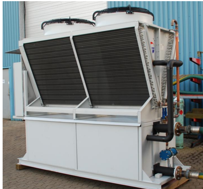
Photo. 6: An inverter driven, screw, air-cooled Propane [R290] chiller on test.
