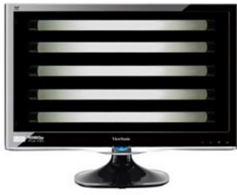
Cold Cathode Fluorescent Lamp
