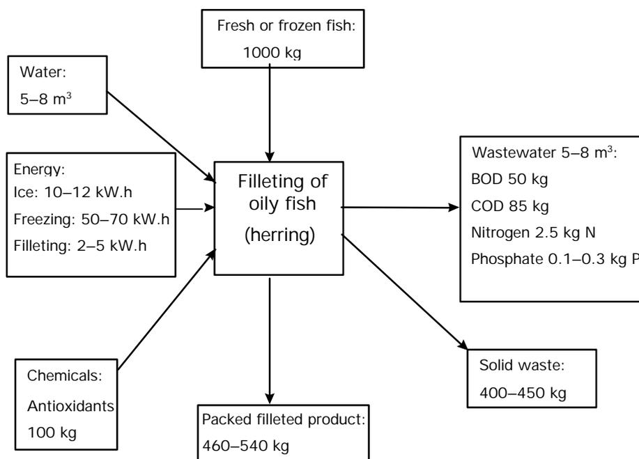
**Figure 2–7 Inputs and outputs for filleting of oily fish (herring) using average technology**
