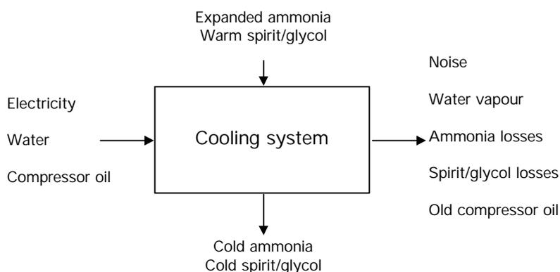
**Figure 3–29 Inputs and outputs for cooling system**
