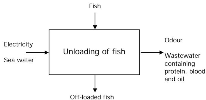
**Figure 3–16** *Inputs and outputs for unloading of fish*
