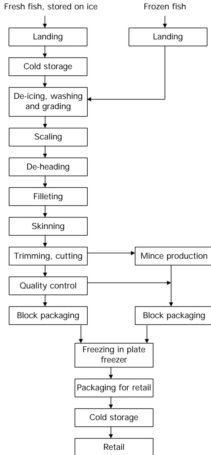
**Figure 2–2** Process flow diagram for the filleting of white fish
