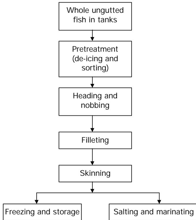
**Figure 4–1 Process flow chart of the operation**
