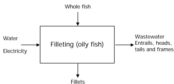
**Figure 3–6 Inputs and outputs for filleting oily fish**
