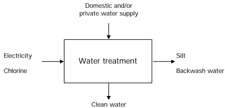
**Figure 3–28 Inputs and outputs for water treatment**
