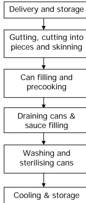
**Figure 2–4** Process flow diagram of the canning process
