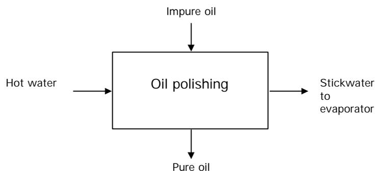
**Figure 3–23 Inputs and outputs for oil polishing**
