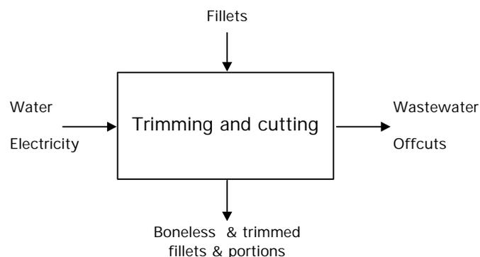
**Figure 3–8 Inputs and outputs for trimming and cutting**
