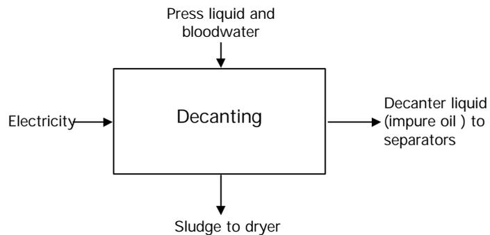
Figure 3–21 Inputs and outputs for decanting of press liquid
