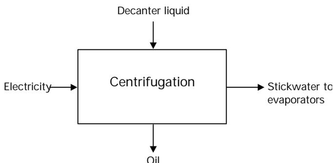
**Figure 3–22 Inputs and outputs for heating and centrifugation**
