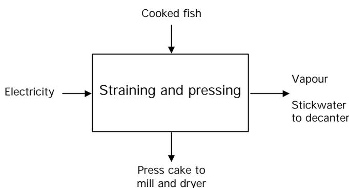
**Figure 3–18 Inputs and outputs for pre-straining and pressing**
