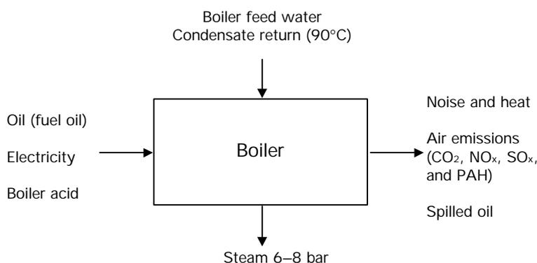
**Figure 3–27 Inputs and outputs for supply of steam**
